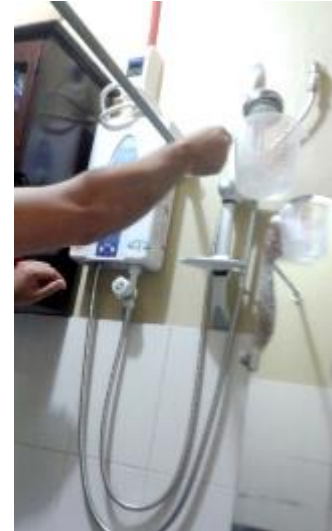
WATER AUDITOR MEASURING THE SHOWERHEAD FLOW RATE
